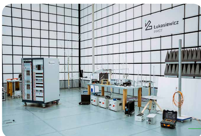
Stand for electromagnetic compatibility testing – EMC chamber
