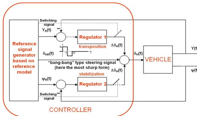
**Figure 4.** Schematic diagram of the lane change control system
