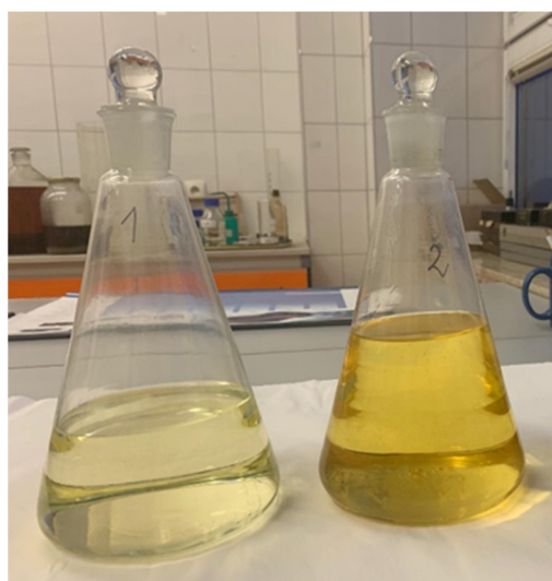
Figure 2. Liquid products from thermolysis of a mixture of plastics (PE, PP and PS): (1) HTG—petrol fraction, (2) HTD—diesel fraction.
